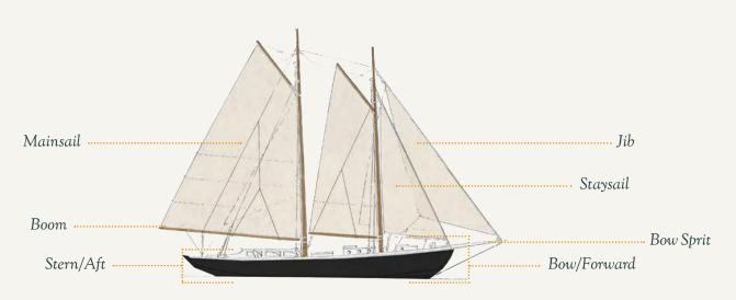
This diagram illustrates parts of a boat only and is not representative of the boat you will be sailing on.
